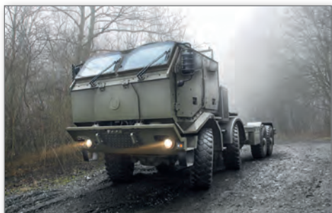
T 815-790R99 38 300 8x8.1R 8x8 HMHD CHASSIS WITH ARMoured DOUBLE CAB Level Level 2 – 2a/2b STANAG 4569
