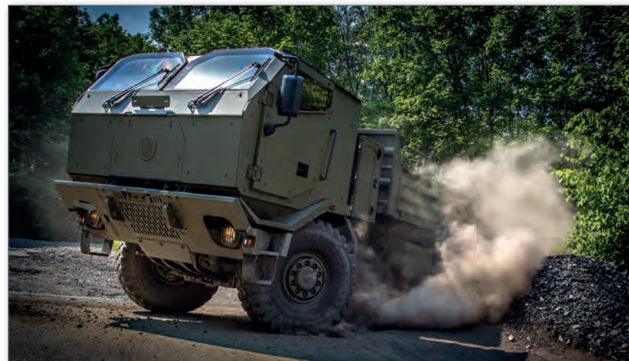
T 815-780R59 19 270 4x4.1R, the first 4x4 logistic truck with armoured cab, which meets Level 3 – 3a/3b according STANAG 4569
